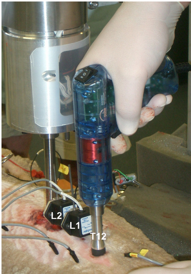
Figure 1 Experimental setup illustrating the Impulse Adjusting Instrument® positioned over the T12 spinous process and the two triaxial accelerometers rigidly attached to stainless steel pins at L1 and L2.
