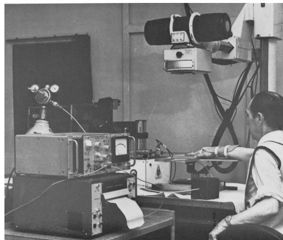
Fig. 2 Experimental setup used to simultaneously measure MCP joint surface separation and applied force. The original caption of this figure, reproduced from Unsworth et al. [10], was “A machine designed to ‘crack’ the metacarpophalangeal joints of human subjects”
